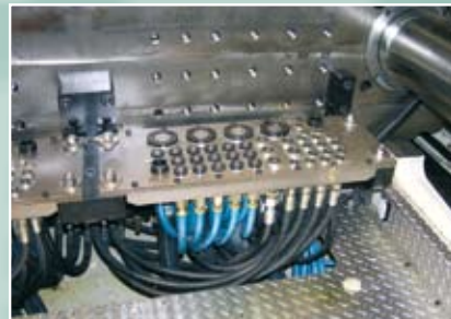
Pneumatic automatic coupler to connect electrical connectors and hydraulic lines in a special machine.
