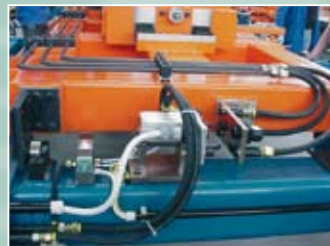
Mold-mounted multi coupler plates.
