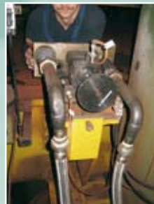
Two large, size 37, couplers to connect cooling lines on a die casting machine. Also suitable in a hot and dirty environment.
