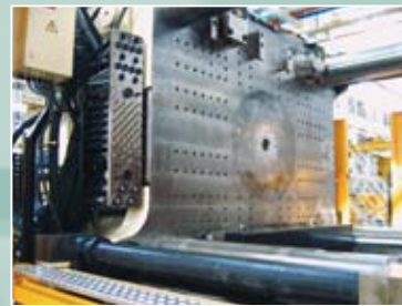
A large automatic multi coupler mounted on the side of an injection molding machine platen with leak-proof connections for water, hydraulics and electrical connections. Hose guides are fitted to support the heavy hoses properly.
