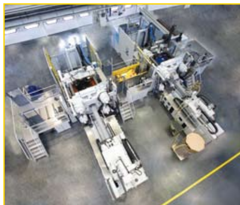
A 15t mould changed in less than 60 seconds
