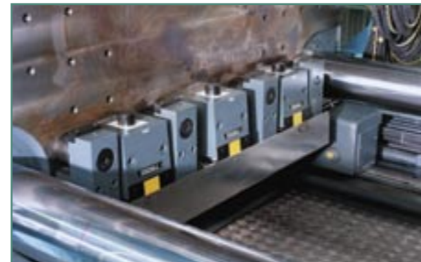
Each machine is equipped with self-locking adaptive hydraulic clamping and rollers for quick and easy horizontal loading and clamping of the moulds.
