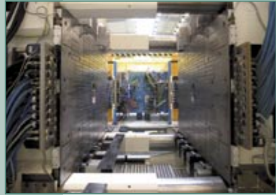
Magnetic clamping system, powered rollers for fast mould movements and automatic multi couplers for leakproof connection and disconnection of the cooling, hydraulic and electrical connections in a few seconds.
