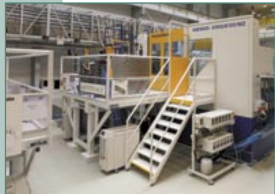
Mould change tables for 1000 t KM machines for fast and flexible production, equipped with powered rollers and multi couplers to preheat and cool the large moulds.
