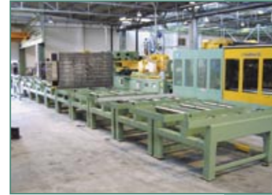
On the other side of the rail guide car are 9 mould storage systems, on which the moulds are stored using the mould change car.
