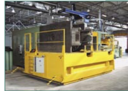
The rail-guided mould change car for two moulds of max 50 t. This car can be operated by means of a remote control unit and is equipped with steps for easy access to the top of the car, as well as safety bumpers.
