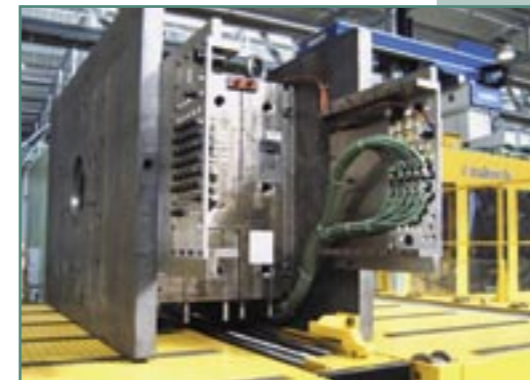
Each mould has standardized backplates and is equipped with standard automatic multi coupler plates on which water, hydraulic and electrical connections are gathered.
