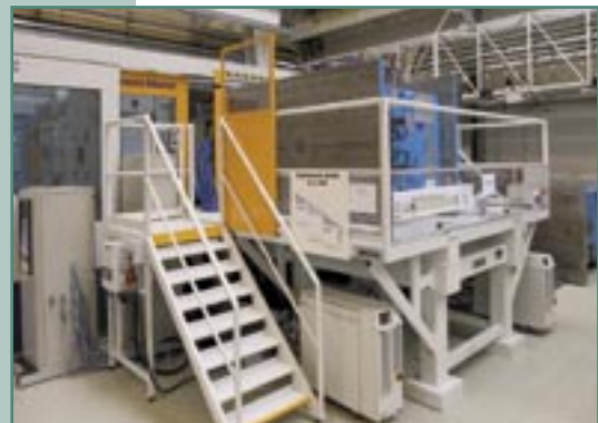
Mould change table with powered rollers and automatic preheating and cooling multi couplers on a 2700 t Krauss Maffei injection moulding machine.
