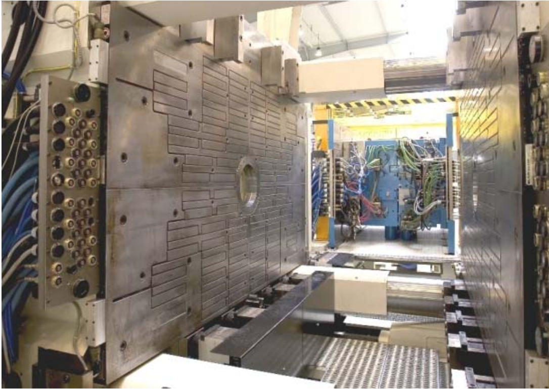
Fig. 11: EAS magnetic clamping system as part of a fully automatic mould change system (side entry of injection moulds) on an injection moulding machine with 3200 tons clamping force.
