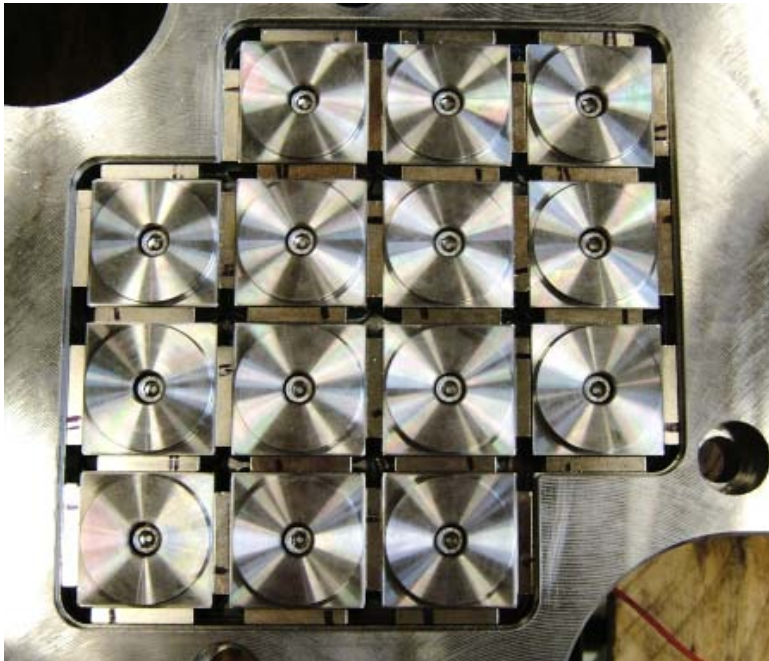
Illustration 2: The new Pressmag SP 100 Permanent Electro-magnetic Clamping unit from EASchangesystems is ideal for standard-size injection moulding machines up to 400 ton capacity and operating in temperatures of up to 100° C. It features the small, 47 mm square pole design and resin sealing. (Photo: EASchangesystems)
